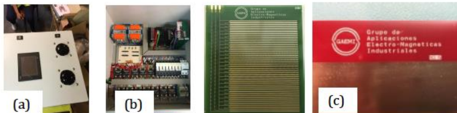
Electroportation (a) External view of the electric generation prototype. (b) Electronics inside the prototype. (c) Electroportation screens in pcb.
