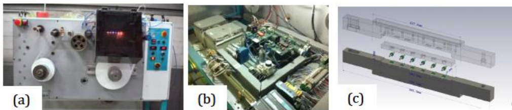
(a) Electroperforation System designed by GAEMI. (b) Electronics inside the prototype. (c) Circular electrodes scheme for electroportation
