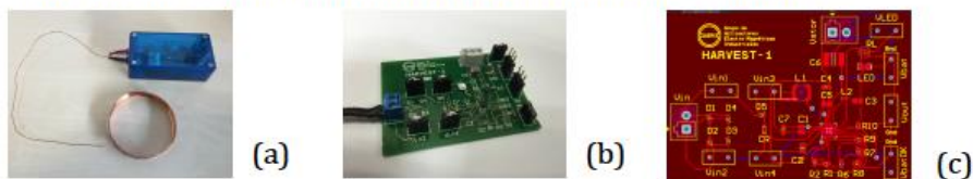
Harvesting system (a) external view (b) pcb picture (c) layout scheme.
