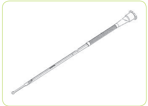
► Fig. 1. The devise comprises a portion for loading the embryo, a channel arranged for conducting a warming solution, a handle portion and a connector for connecting the device to the warming solution source.
